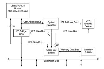
Figure 2. Uniprocessor System Configuration
